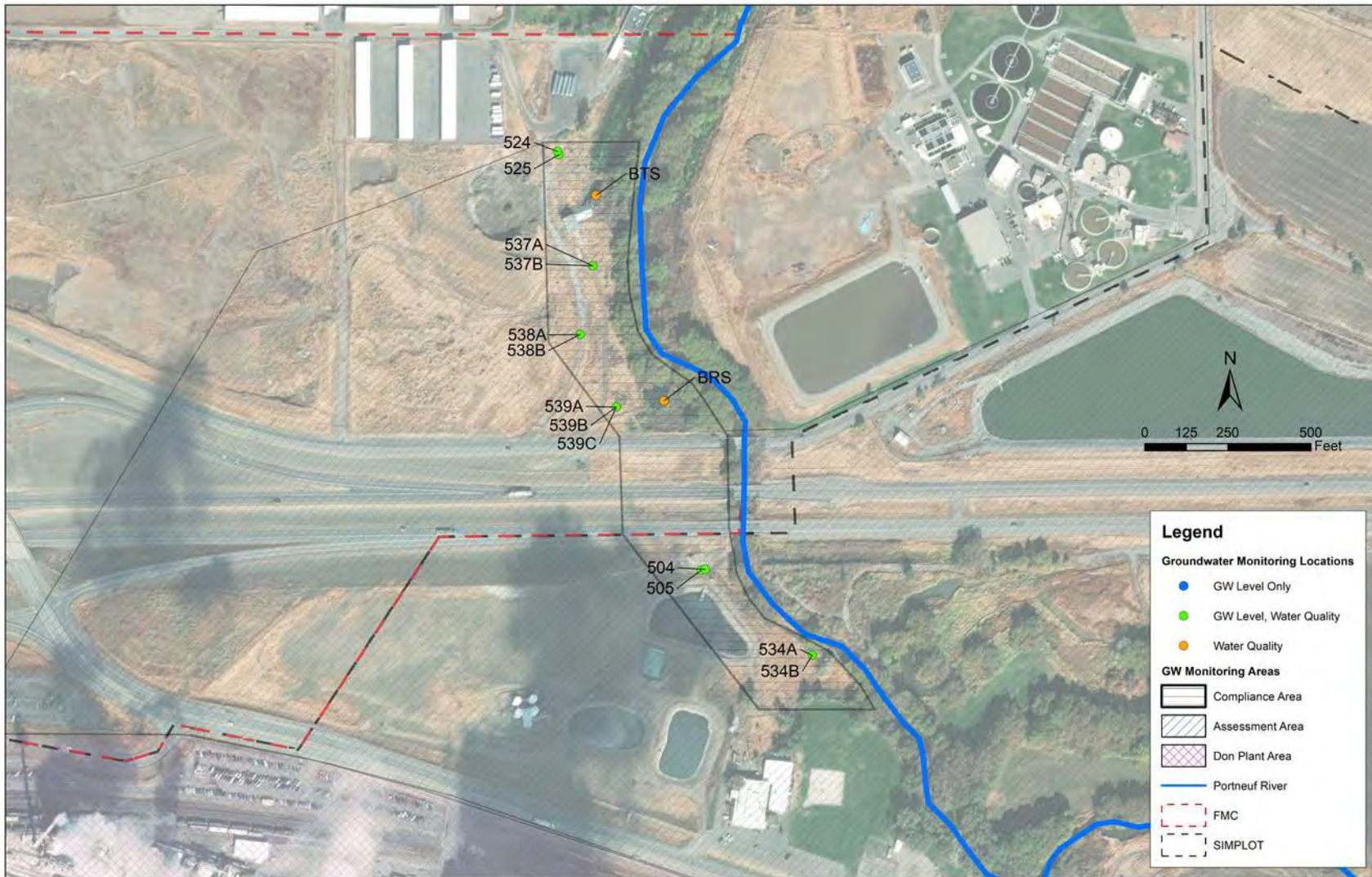
Figure 2-5: Monitoring Locations in the Compliance Area
