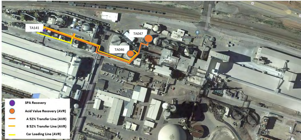
Figure 9: Acid Transfer between the Phosphoric Acid Plant, Truck and Rail Loadout, and SPA Evaporator Feed Tank 17
